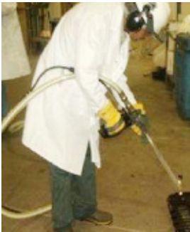
A dry ice "blaster" is used to clean various parts of our Chanhassen, Minn., facility. This has not only resulted in a reduction in employee cleaning time, but also a reduction in use of water and cleaning chemicals that would have been discharged to the sanitary sewer.
