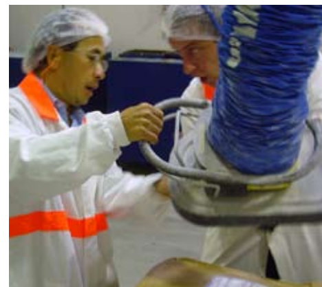
We have started to use vacuum-assisted lifting devices to move heavy bags of ingredients at our Rooty Hill, Australia, plant.
