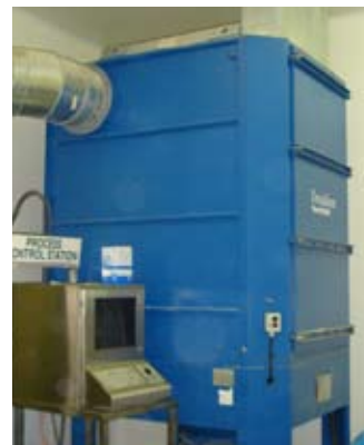
This small dust collector at our Berwick, U.K., plant is used for collecting dust from food materials.
