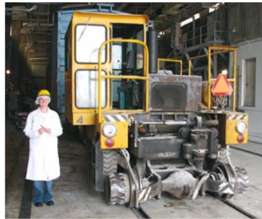
One of our divisional safety managers is shown after inspecting a "Trackmobile," which is used to safely move railcars at many of our manufacturing facilities.
