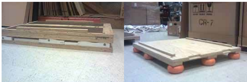
Replacing one layer of a typical wooden pallet with doughnut cushions saves about 30 kilograms per crate.
