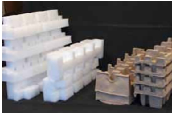
Expanded polyethylene and molded pulp cushions
