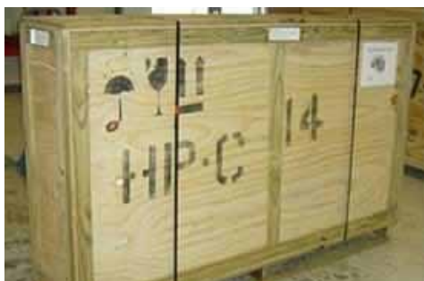
Transitioning from a wood crate to a cardboard crate saves more than 20 kilograms per crate. About 14 crates are included with each system.
