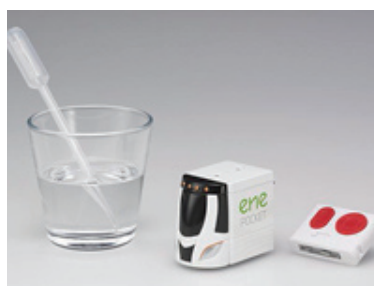
Toy car with glucose-powered remote control
