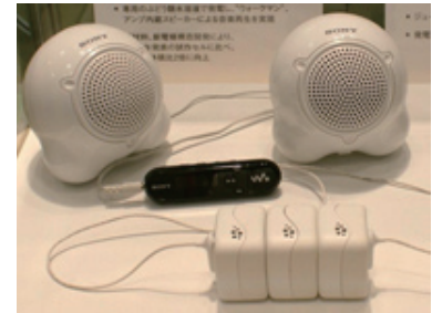
Powering a Walkman digital music player using a prototype bio battery that generates power from a glucose solution (February 2009); this new prototype is half the size of the previous prototype.
