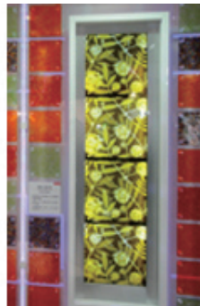
Power-generating window prototype that incorporated dye sensitized solar cell was integrated with energy storage module in the demonstration of "Room of the Future" concept ("ECO PRODUCTS Exhibit 2010" in December 2010)
