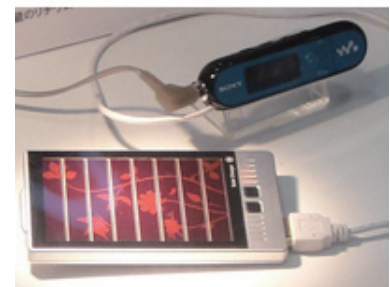
Demonstration of the use of a prototype dye-sensitized solar cell/Li-ion battery hybrid charger to power a Walkman digital music player (December 2009)
