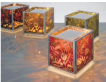
Demonstration of Hana-Akari, a concept model of a lantern-like interior lamp powered by colorful, see-through dye-sensitized solar cells (December 2008)
