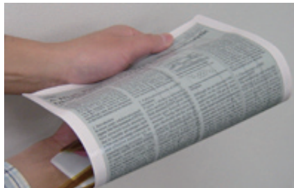
Organic TFT-driven flexible electronic paper produced using coating technology (May 2011)
