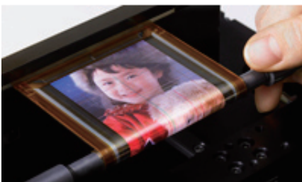
An organic TFT-driven EL display capable of video playback while being rolled up to the size of a pen (May 2010)
