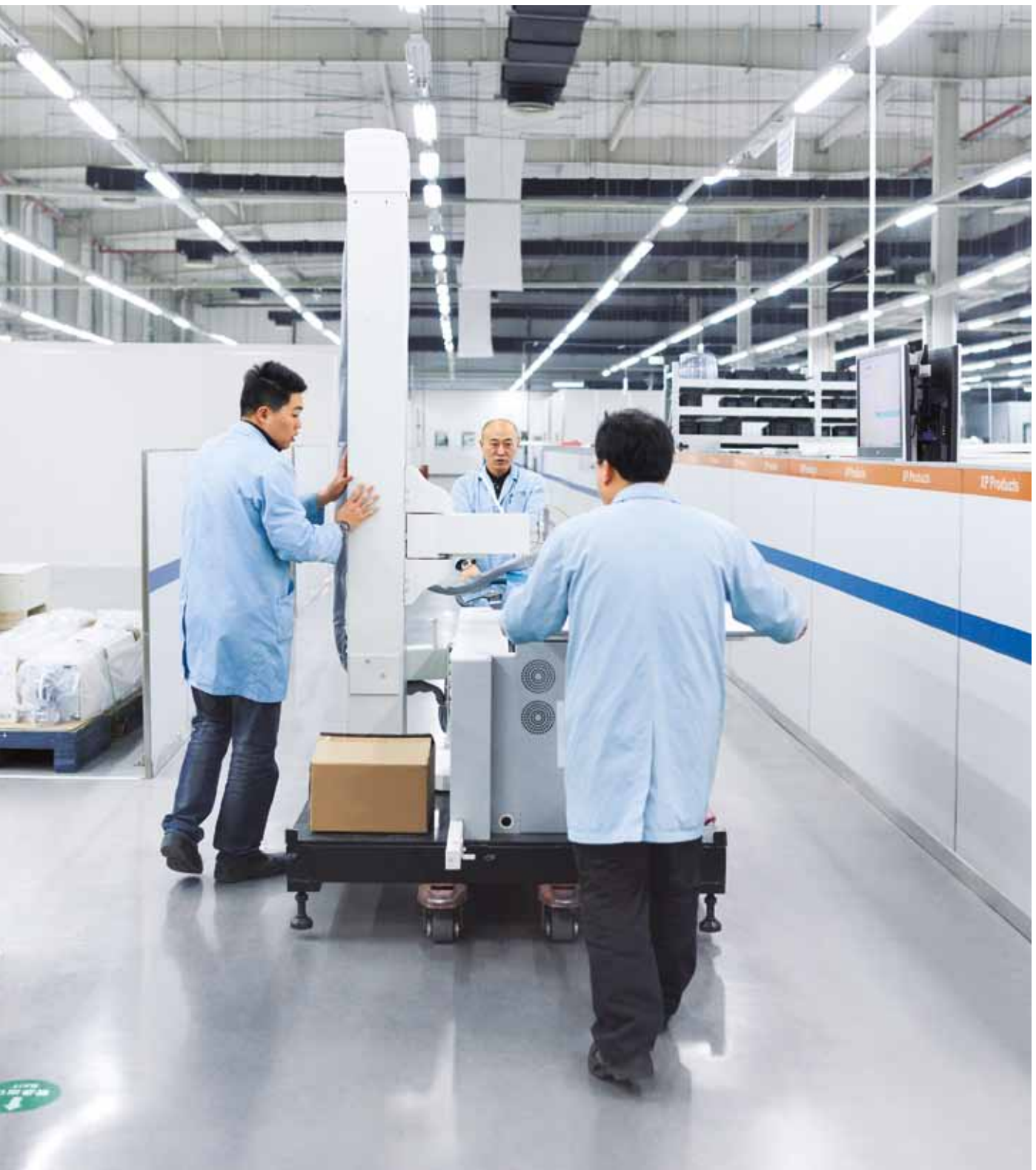
ABOVE – On site in Shanghai: the individual components are picked for shipment and preassembled by our technicians.
