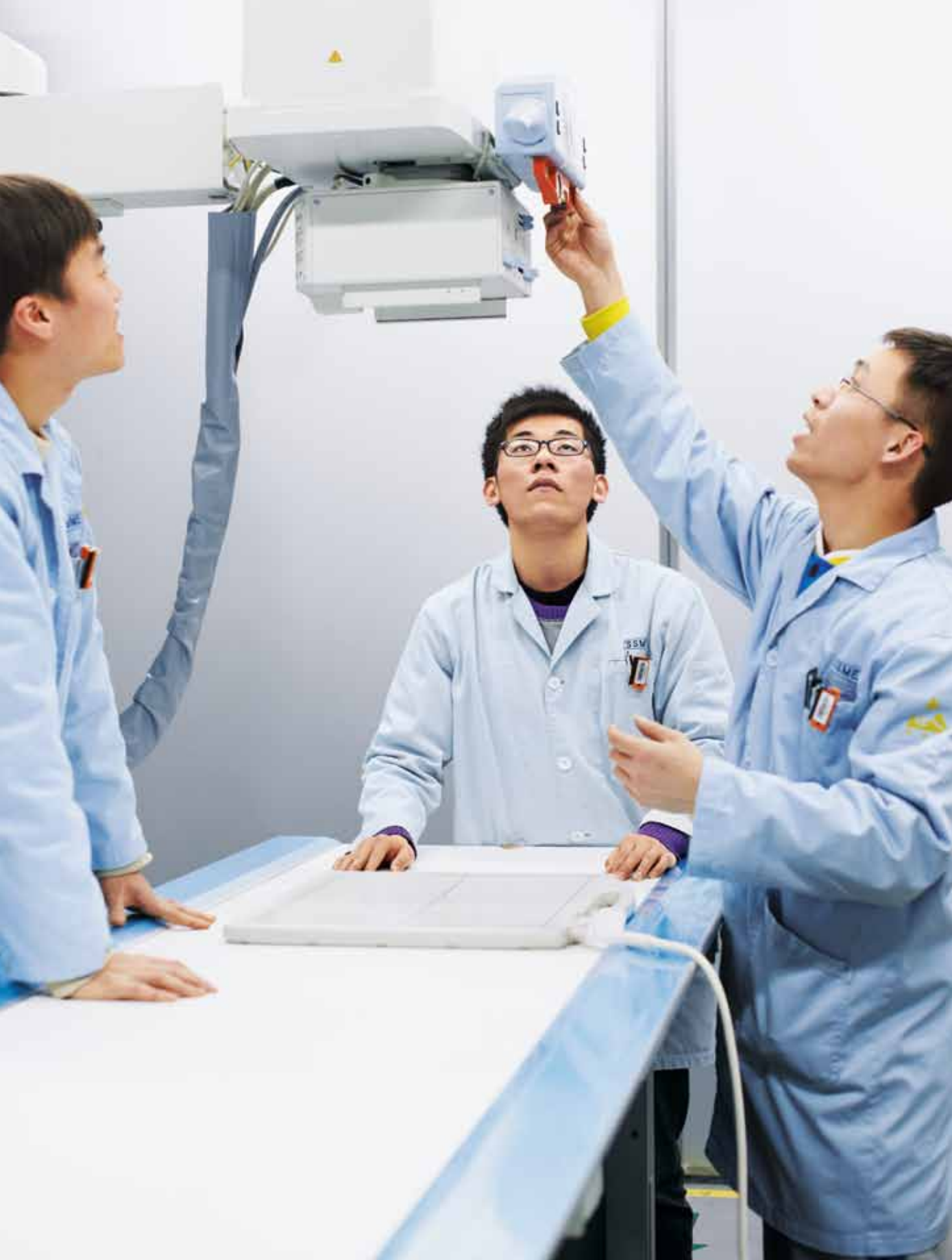
ABOVE – Before delivery our engineers inspect the technical reliability and image quality of the Multix Select DR. The mobile X-ray detector can be seen on the X-ray table.
