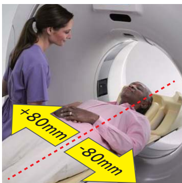
Multi-slice CT system table that slides from side to side
