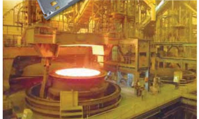
Electric furnace at Tokyo Steel
