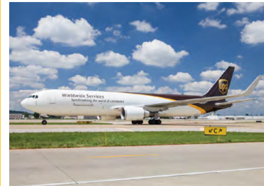
Boeing 767 with customized winglets
