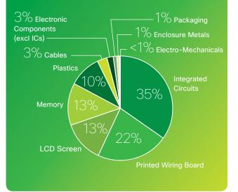
of a Cisco IP Phone. The largest impact areas identified in this phase (integrated circuits, bare printed circuit boards, displays, and assembly and test processes) are also the most challenging to collect accurate data for modeling. To address this challenge, Cisco is working with industry peers and suppliers to collect more data and improve calculations.
