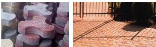
Road pavement blocks made of foundry waste sand and road paved with the blocks
