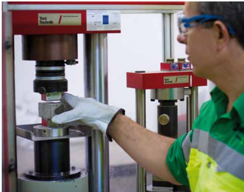
Compression test of cement by qualified personnel in the plant lab
