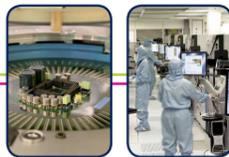
We electrically test the die on the wafer. It is also known as wafer sort or probing.
