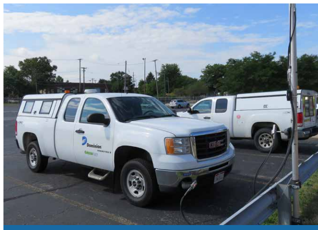
Photo: The use of CNG in light-duty pickup trucks requires about 90 percent less gasoline than regular gasoline-fueled, light-duty pickup trucks. In 2015, our CNG vehicle fleet displaced the equivalent of more than 200,000 gallons of gasoline.
