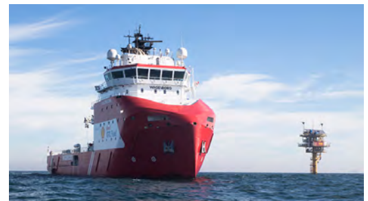
Kronborg is the first offshore vessel in the world to sail on GTL fuel, a liquid fuel made of natural gas with less emissions than conventional fuels for vessels.
